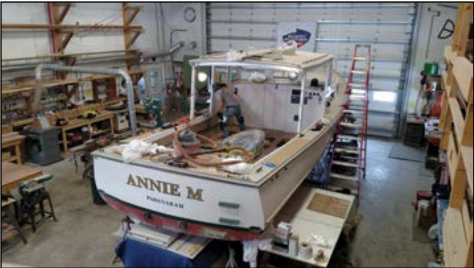
This is an older Holland 32, which was purchased last fall and found to have some deck issues caused by moisture staying in between the platform and the Soundown. She was brought to Belmont Boat Works in Belmont where her platform was removed and they are now in the process of replacing it.
