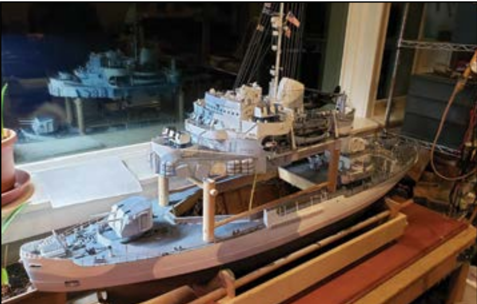
This is a RC model of the icebreaker USS EASTWIND built 1943-4 in Arctic camouflage, which operated around Greenland during World War II. The hull is plank on frame and covered with fiberglass and the superstructure is scratch built with a number of 3D printed parts. This model took about three years to complete.
