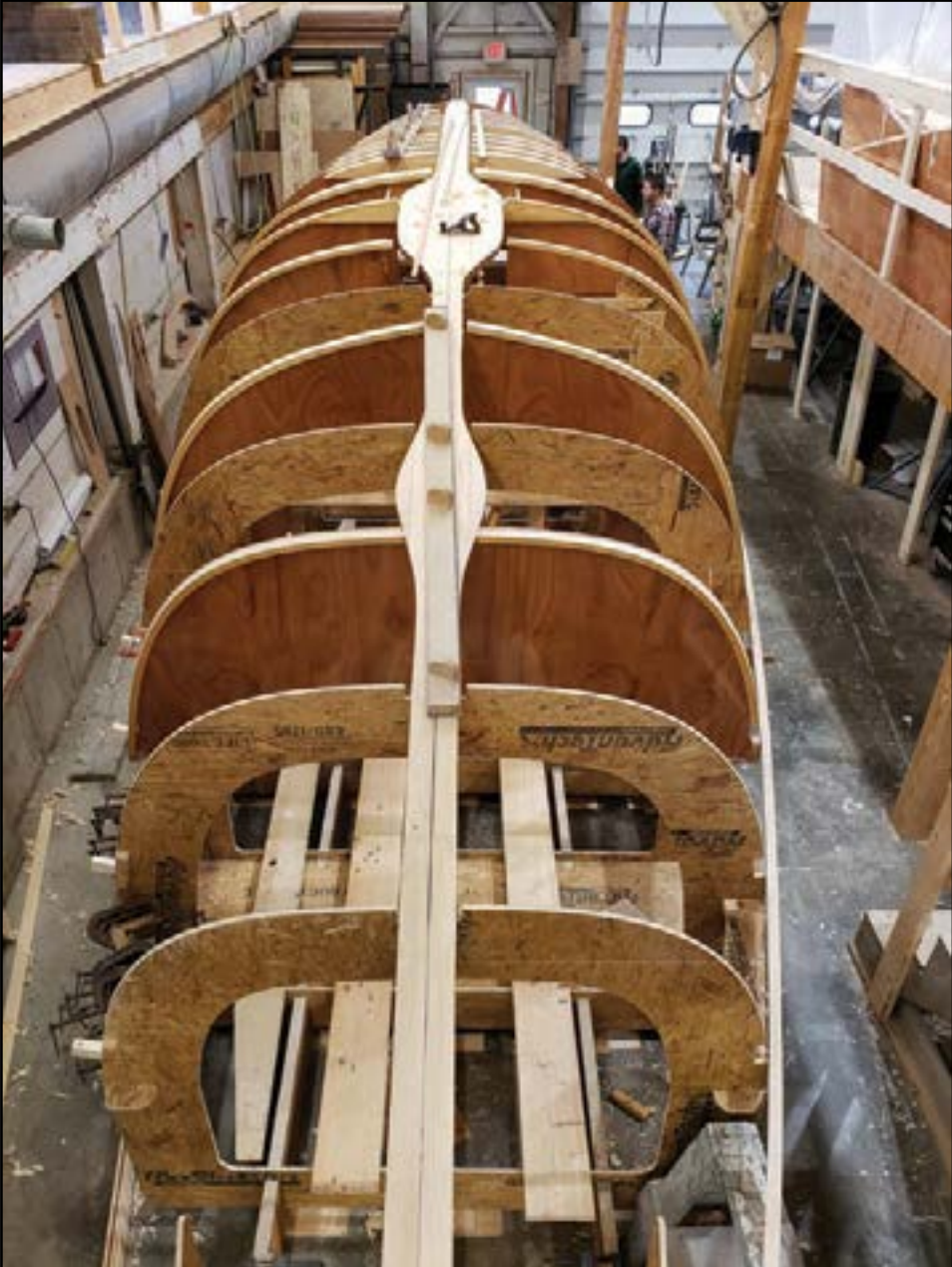
The Jim Taylor designed 50-footer is being set up just to the right of the Wheeler at Brooklin Boat Yard in Brooklin. You can see that her bulkheads and back-bone are in place. She is being finished off for a local customer.
