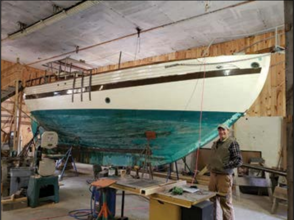
At Buxton Boats in Sunset we caught Peter Buxton working on the x-MARION D., which is a Colin Archer designed and Norwegian built sailboat. She went in this past summer after being out of the water for a number of years and she developed a noticeable leak. Peter has removed the garboards and will take a closer look at the ribs and keel bolts, but felt that the real problem was the caulking.
