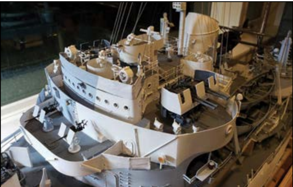
This is a RC model of the icebreaker USS EASTWIND built 1943-4 in Arctic camouflage, which operated around Greenland during World War II. The hull is plank on frame and covered with fiberglass and the superstructure is scratch built with a number of 3D printed parts. This model took about three years to complete.
