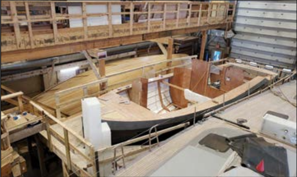
At Brooklin Boat Yard in Brooklin work is progressing well on the 39-foot Wheeler pleasure boat in the middle and the Jim Taylor designed 50-footer, which you can see they are putting the layers down on her cold moulded hull.
