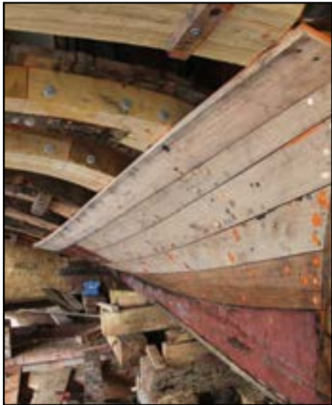
A view looking forward showing the stern post, which has been replaced along with a number of frames and planks on the Rock-land schooner STEPHEN TABER.
