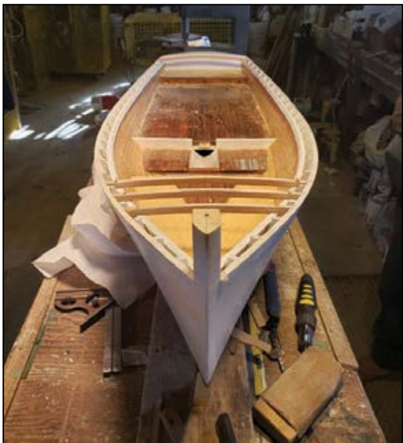
At Willis Beal’s Boat Shop on Beals Island he has another model underway this winter. This is a model of SPRUCE III and as you can see the hull is done and he is working on the deck.
