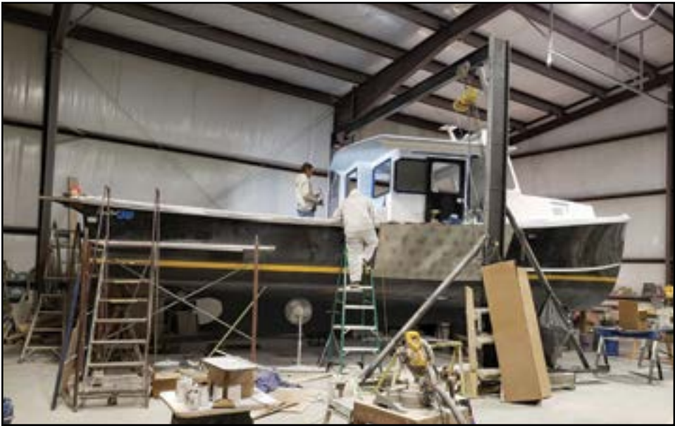
At Friendship Boat in Friendship they have nearly completed this Wayne Beal 36, which is being finished out as a lobster boat for a local fisherman.
