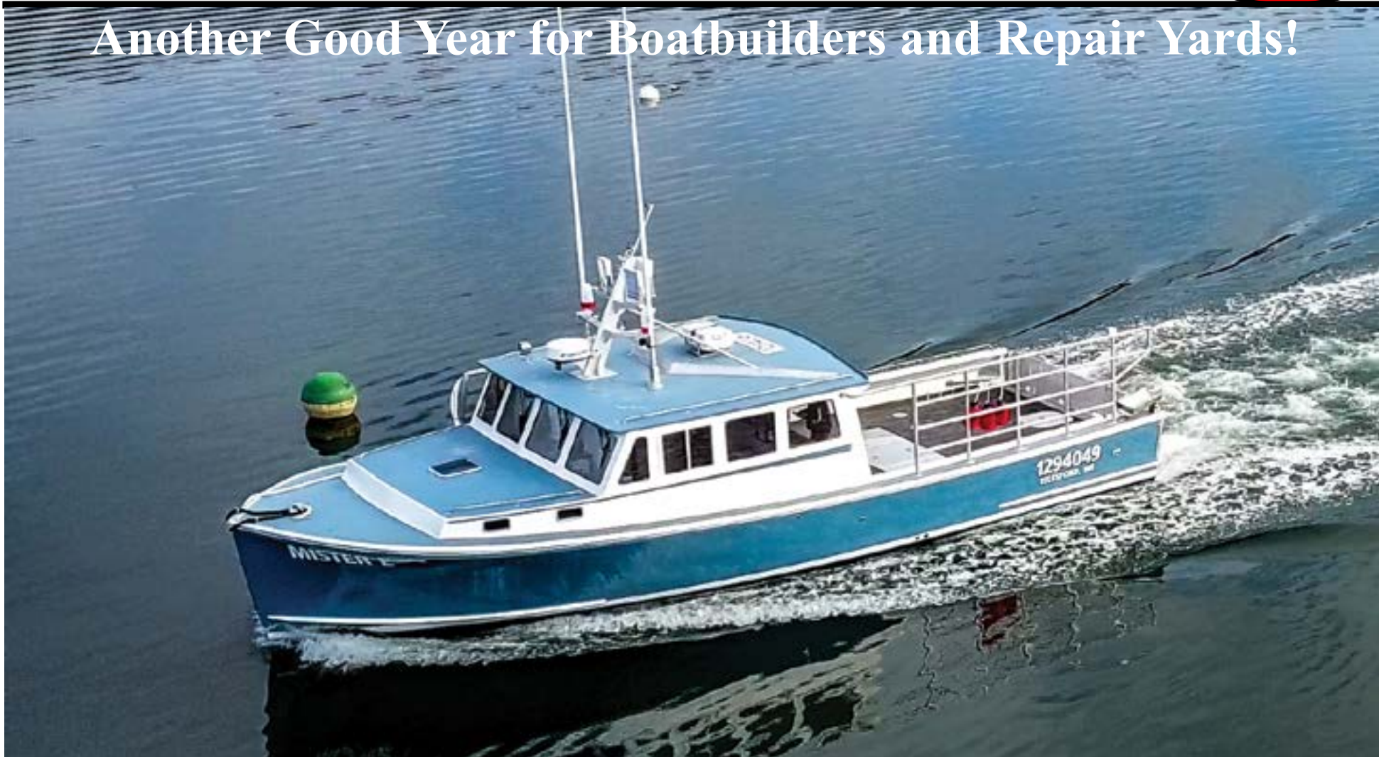
MISTER E., a Calvin Beal 44, finished off as a lobster boat for Nicko Hadlock of Cranberry Isle by S. W. Boatworks of Lamoine. She is powered with a 750-hp John Deere, with a 2.48:1 gear, and reached a speed of 23 knots.
