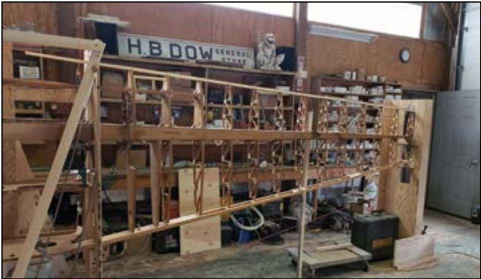
At Eric Dow's shop in Brooklin they are building an airplane. This is a wing, which was built by the owner, but the rest will be completed at Eric's shop.
