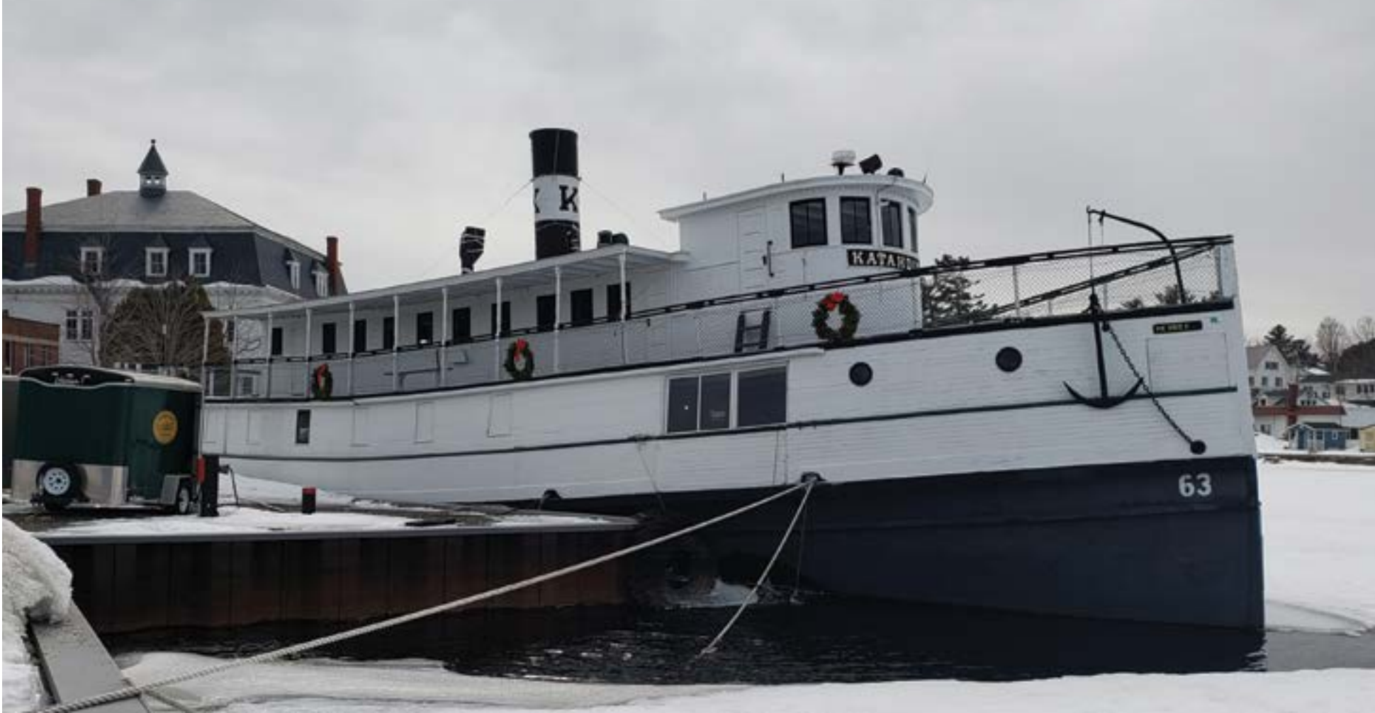
KATAHDIN sitting at her dock on Moosehead Lake in Greenville. You can see that the bubbling system keeps the ice away from the hull even in the extreme depths of winter.
