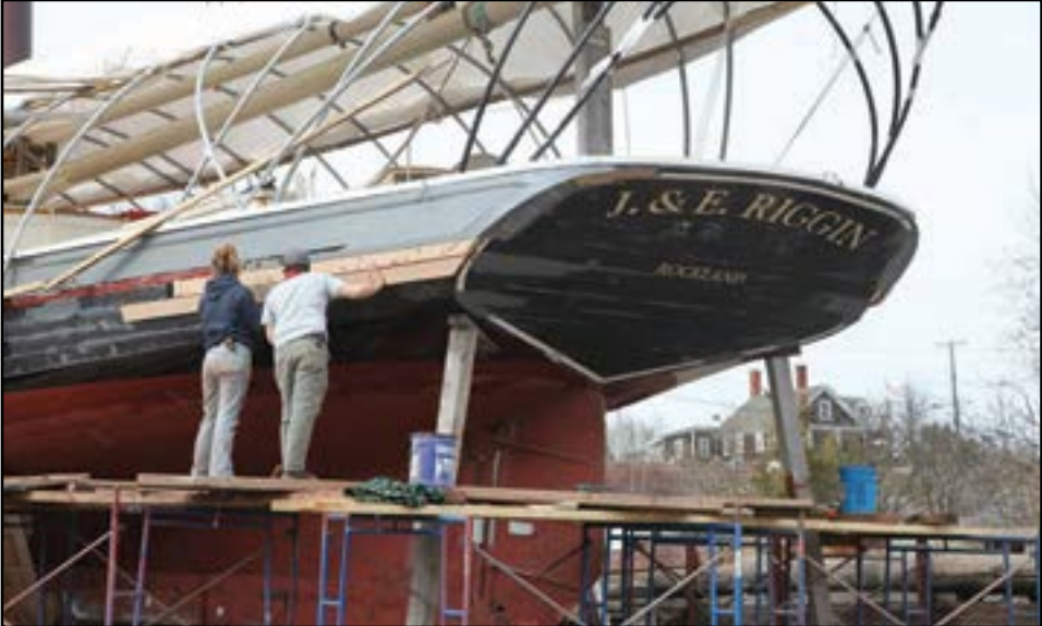
Putting in a couple of new planks on the Rockland schooner J. & E. RIGGIN at Northend Shipyard in Rockland.
