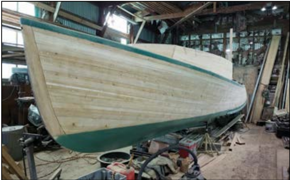
On Beals Island Doug Dodge is progressing on his new race boat, which is 29 feet long with an 8 foot beam. She presently has a 350 Chevy, which he thinks will push her along at 42.
