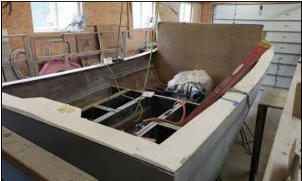
At Sargent Boats in Milbridge they are finishing off this Mitchell Cove 32, which has had her sheer raised 3 inches. She will be finished off as a sportfish for a customer from Newburyport.
