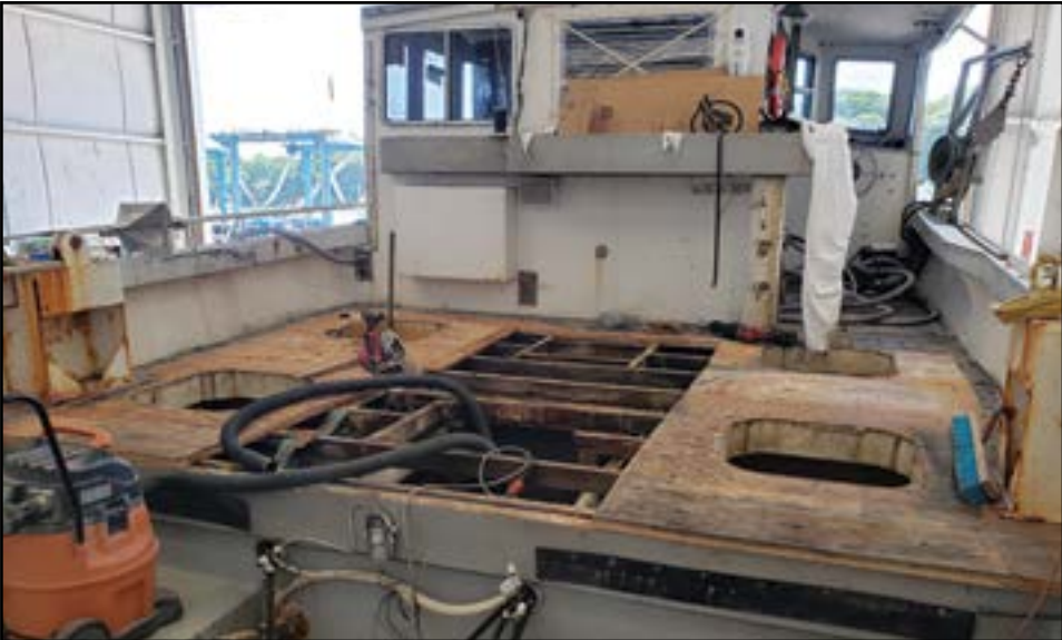
The Newman 46 ERICA JADE from Harpswell hauled up at Royal River Boat Yard in Yarmouth due to a fuel tank leak. She is having her platform ripped out and tanks replaced.
