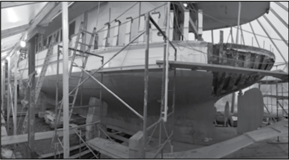
The sardine carrier PAULINE hauled up on the railway at Billings Diesel & Marine in Stonington, where she is getting extensive hulls repairs done by Clark & Eisele.
