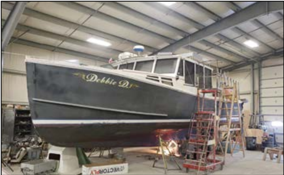
After striking a ledge off Jonesport DEBBIE D. was brought into Wayne Beal Boat Shop in Jonesport for repairs. They have removed 16 1/2 feet of her keel and repaired other damage inside the hull. She will be done late this winter.
