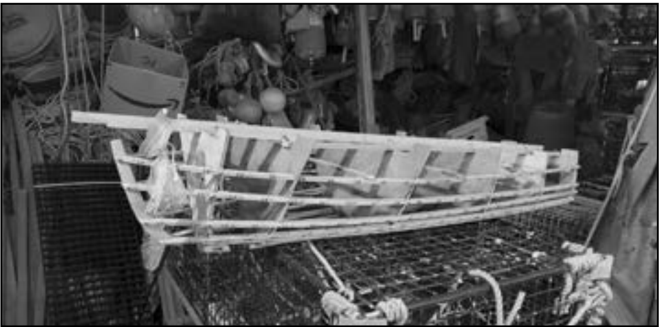
This is a photograph of the jig, which is upside right. You can see the strongback on top with the stations attached and the top ribband would be the position of the top plank. Also, not there are marks on the ribbands and that is where the frames go.
