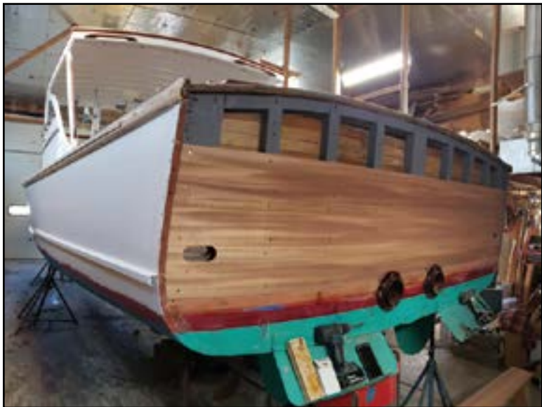
This is the transom of the 34-foot Bunker & Ellis being replaced at Eric Dow's boat shop in Brooklin. It was single planked, but they decided to double plank it so it was more stable.
