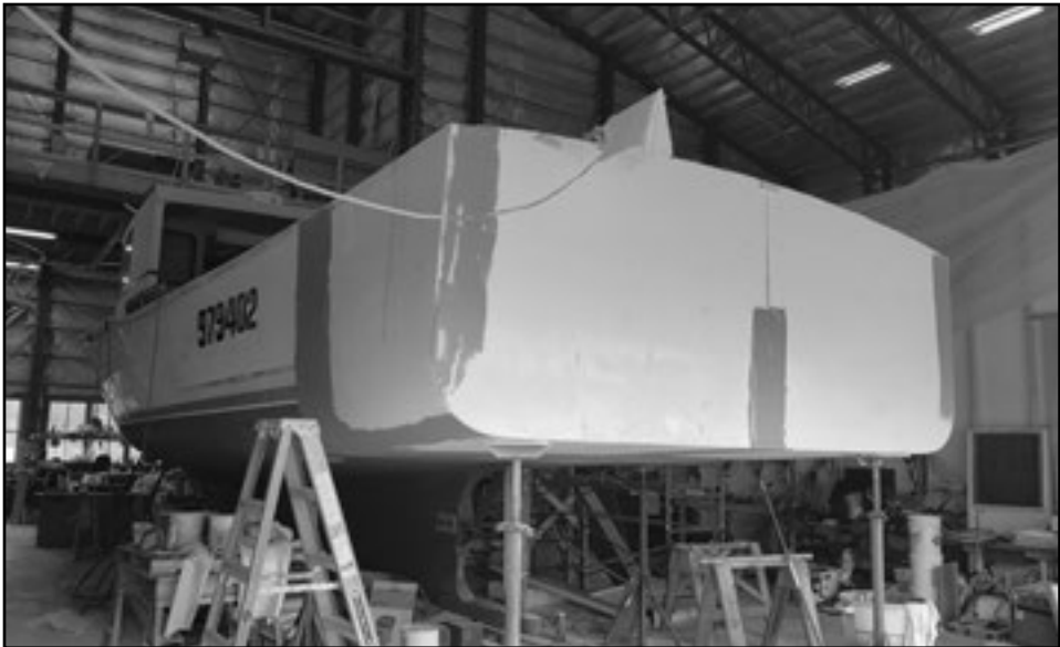
At Gamage Shipyard in South Bristol they have extended the stern of an Osmond 42. They cut pieces out of the turn of the bilge and added a little tumblehome.
