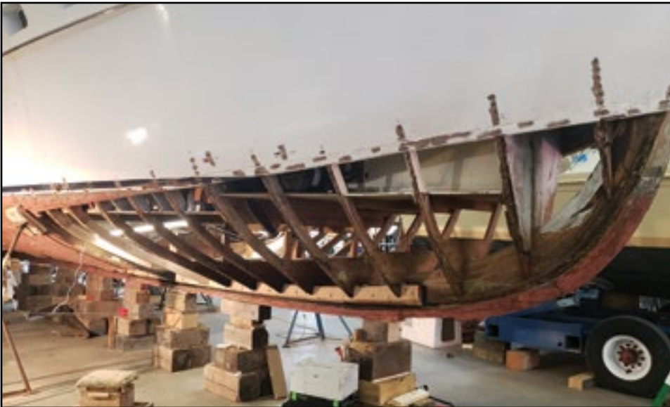
The 55-foot motor yacht having her bottom replaced at Portland Yacht Service in Portland. This project will be finished sometime this summer.
