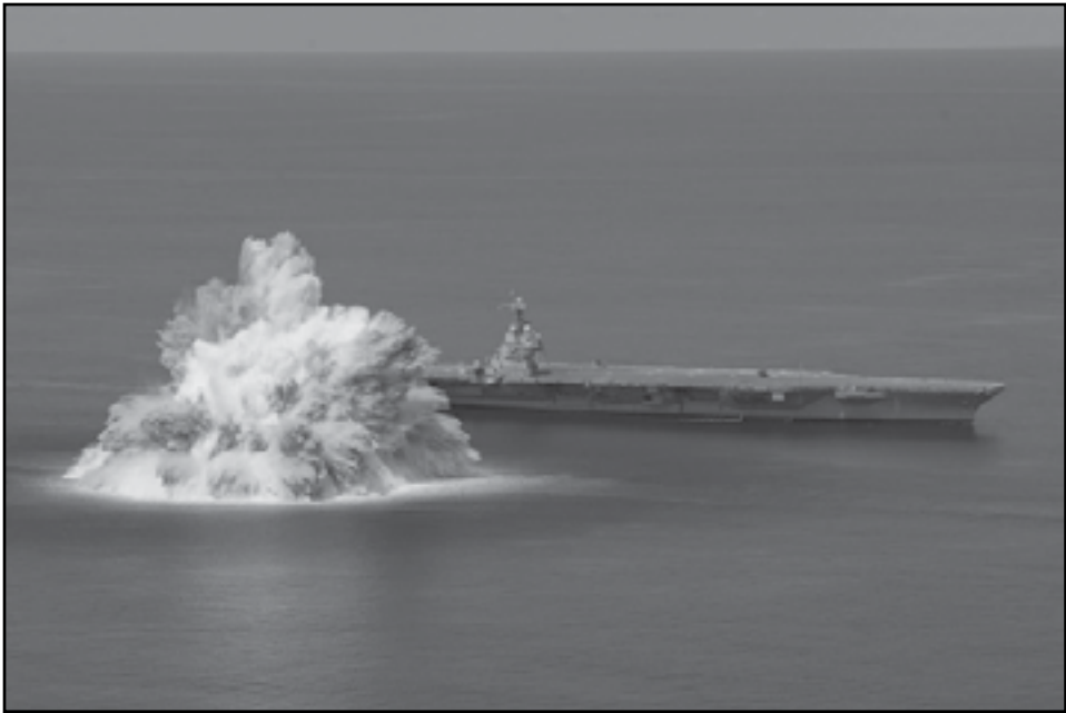
On Friday, June 18, the USS Gerald R. Ford (CVN 78) successfully completed the first scheduled explosive event as part of Full Ship Shock Trials (FSST).
