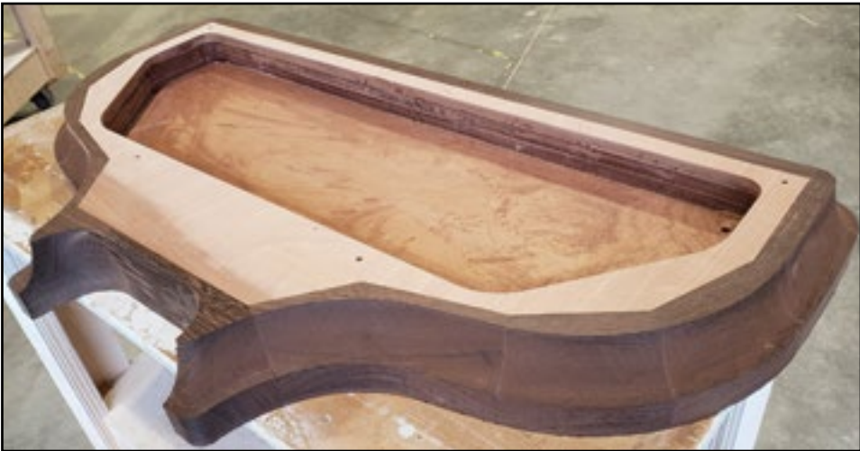
This is a base of a table cut out with a CNC Machine at Hewes & Co. in Blue Hill.
