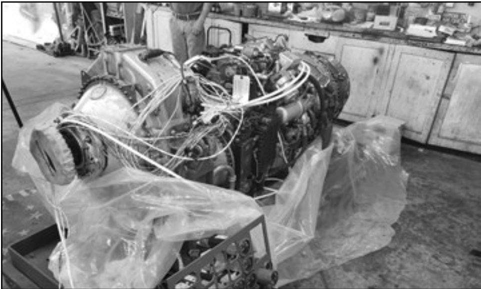
This is the 2,350-hp turbo-prop engine that Steve Johnson of Long Island will be putting into a Crowley-Beal 33. They figure she will not be ready until next spring.
