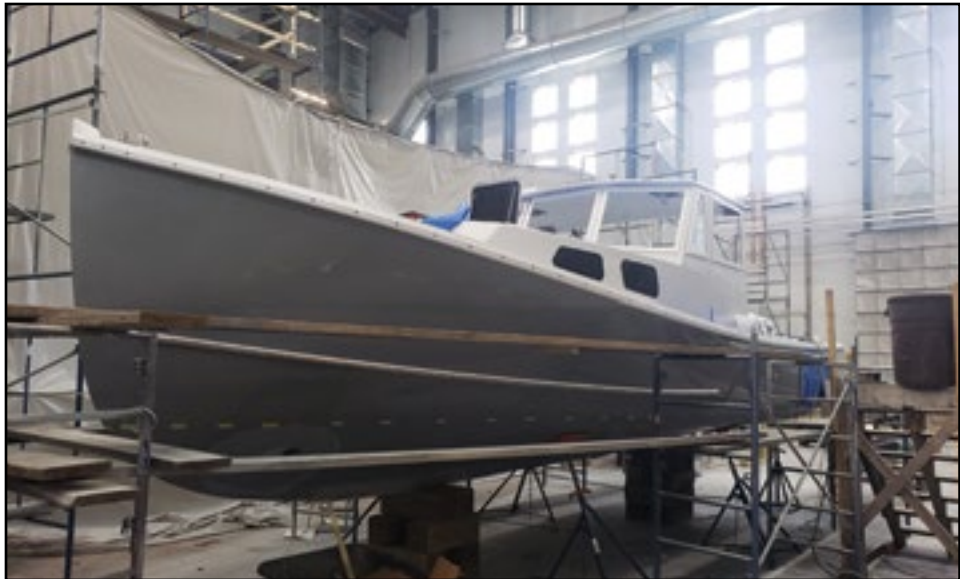
This is a Holland 30 being finished by Front Street Shipyard in Belfast. She will be powered with an outboat and should be in the water mid-September.
