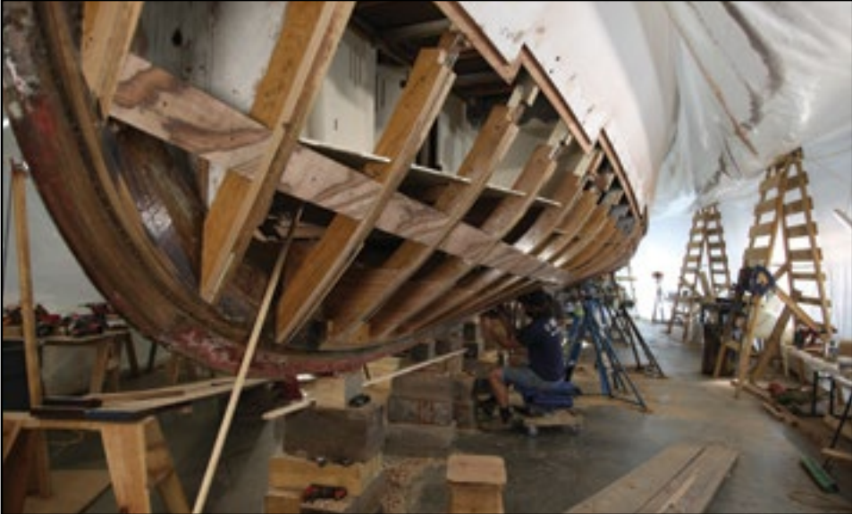
A look under the tarp of the 55-foot Grebe getting a new bottom at Portland Yacht Services. They are fairing the frames so all the planks fit properly.
