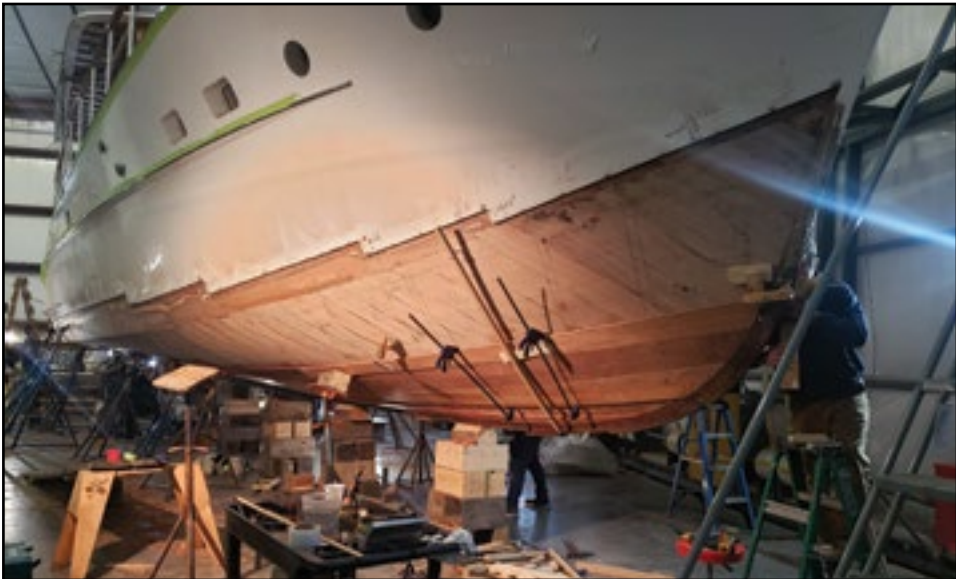
Replacing the bottom on the 55-foot Grebe IROQUOIS at Portland Yacht Service in Portland.
