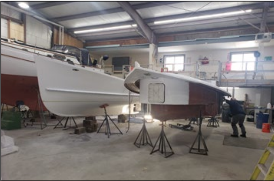
At Atlantic Boat in Brooklin they were getting ready to marry the hull and deck of this 31-foot launch after the Coast Guard their blessing. This one will be going to the Portland Yacht Club in Falmouth.
