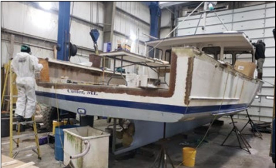
Deep Cove Marine Services in Eastport has a Libby 41 lobster boat in from Cutler for an extension on her stern.
