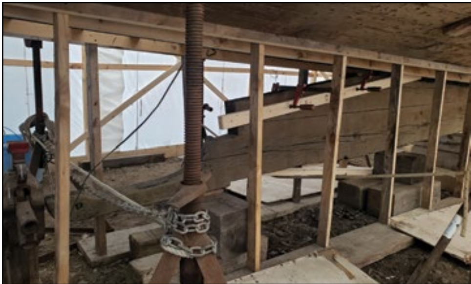
A view of the keel, minus the horn timber, of HARPOON, a 1969 Royal Lowell designed and built cruiser, which is being repaired at Downeast Custom Boat in Yarmouth.
