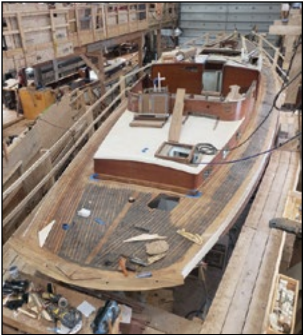
The S&S designed motorsailer DJINN getting a new deck, deck hardware and interior at Brooklin Boat Yard in Brooklin.
