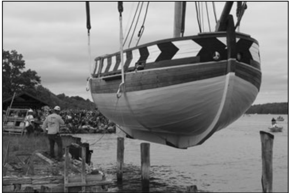
VIRGINIA being hoisted up by two cranes and placed into the Kennebec River at Bath.
