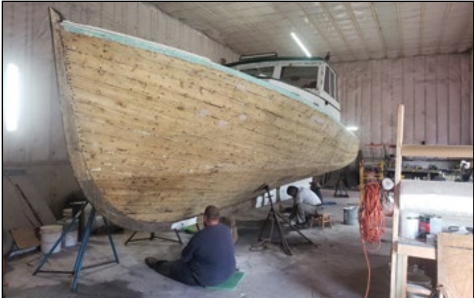
This is a Lowell 36 getting ready to be covered in fiberglass by J. C. Boats of Addison. What they are doing is covering the keel with 5200, which will extend up to the waterline. They will then put a layer of mat on and roll it with a rolling pin. An interesting method.
