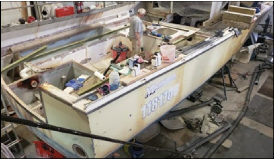
MAGNUM getting a new engine and deck at C. W. Johnsons in Harpswell.
