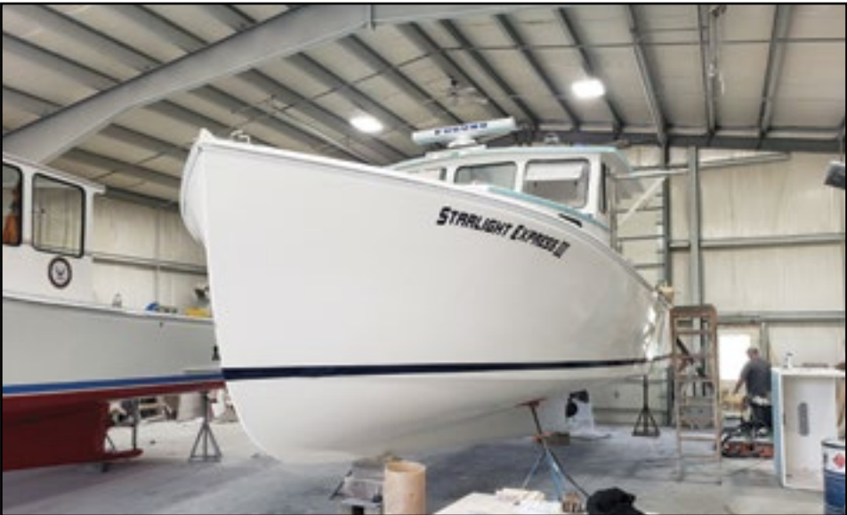
The new STARLIGHT EXPRESS, a Wayne Beal 36 with hard chines, powered with a 1,400-hp MAN, is expected to be in the water the end of the month.
