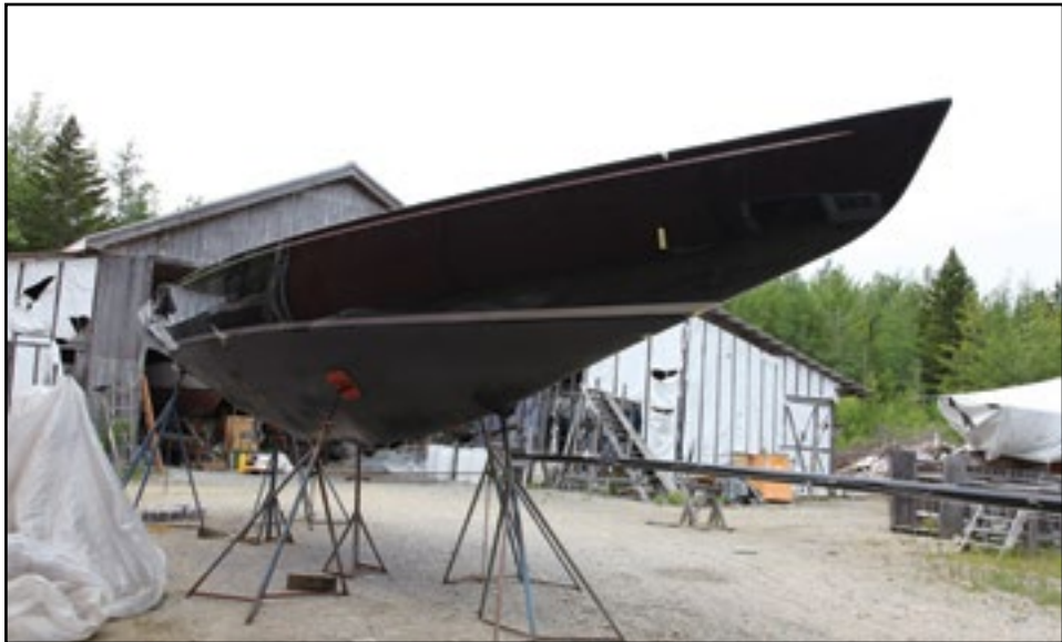
The keel has been removed from this 8-Metre at Brion Rieff's boat shop in Brooklin and will be modified to fit the measurement rule.
