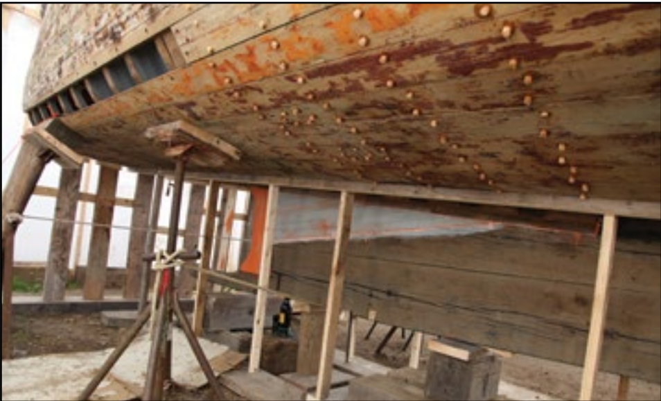
At Downeast Custom Boats in Yarmouth they are making major repairs to this Lowell built cruiser HARPOON. They have wooded the hull, repaired the keel and refastened. There are places that were not refastened, but these are places where they need to add sister frames.
