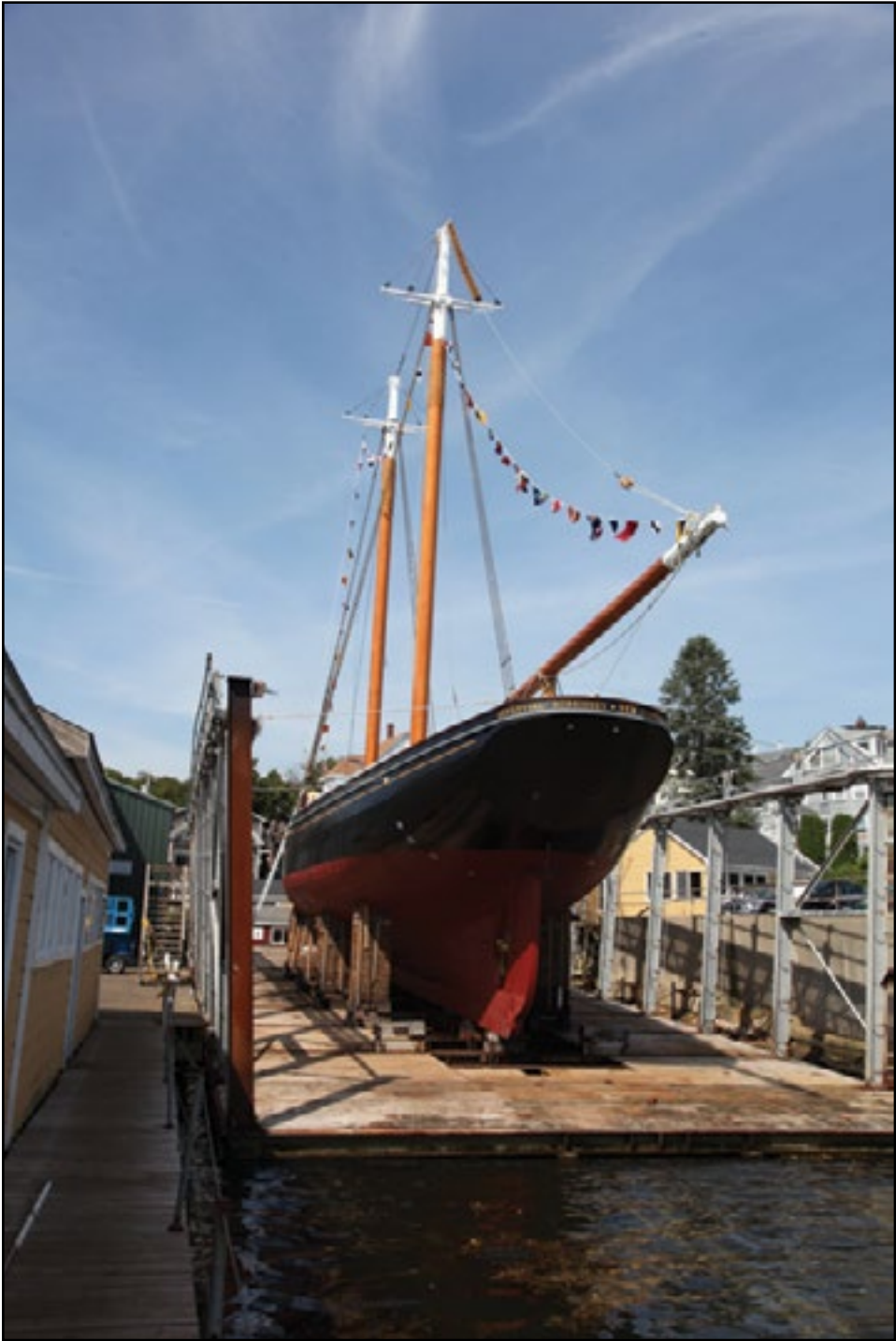
The fishing schooner ERNESTINA-MORRISSEY on the railway at Bristol Marine’s Boothbay Harbor Shipyard at Boothbay Harbor. She has been on the railway several years for a major rebuild and this day they tried to launch her, but developed a problem with the roller boxes and she had to be hauled back up and the roller boxes repaired.
