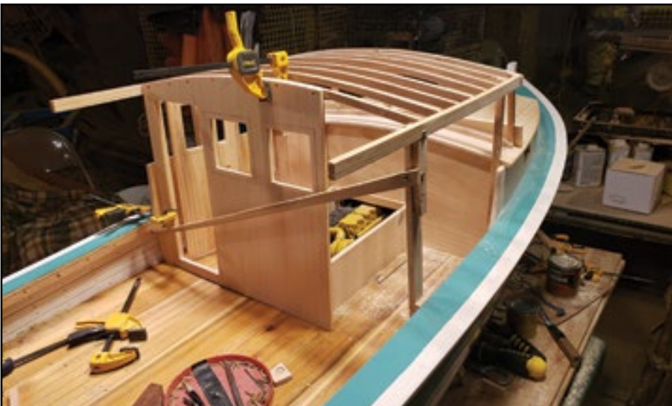
A stern view of the wooden lobsterboat model being built by Willis Beal of Beals Island. Note the details especially the framing for the cabin top and the engine.
