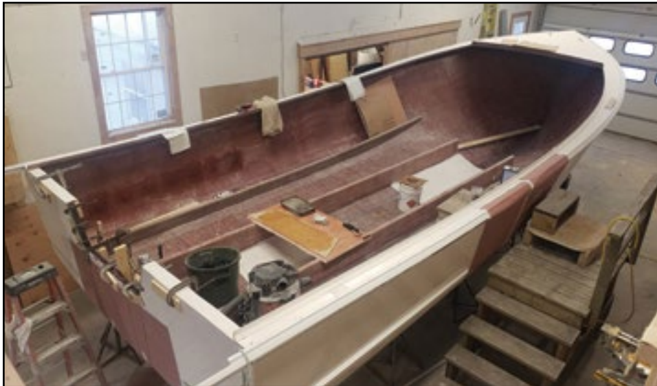
This is a Calvin Beal 30 hull in Eaton's Boat Shop on Deer Isle. She is being finished out as a pleasure boat for a customer who will use her on the upper Hudson River in New York. She will be powered with a 425-hp outboard.
