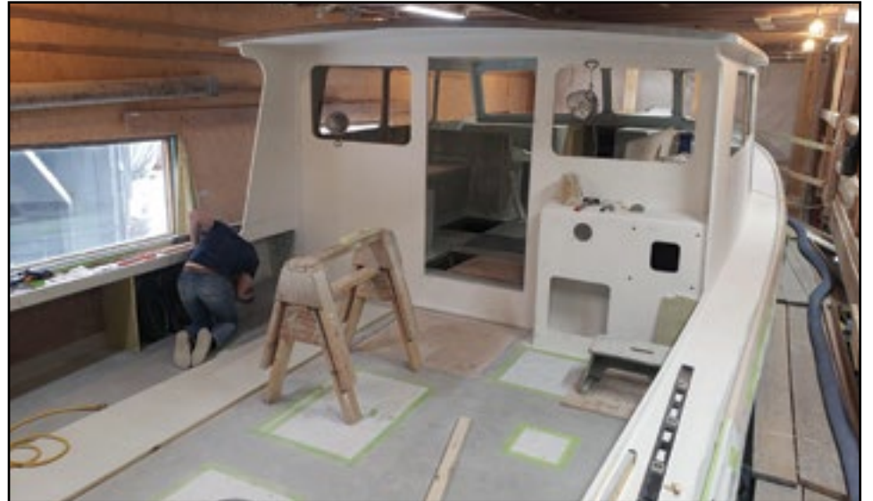
This is a Mussel Ridge 46 being finished out as a commercial/pleasure cruiser for a customer from California by Farrin's Boat Shop in Walpole. She is powered with a C-18 Caterpillar and sports a full interior. She is scheduled to be completed this spring.
