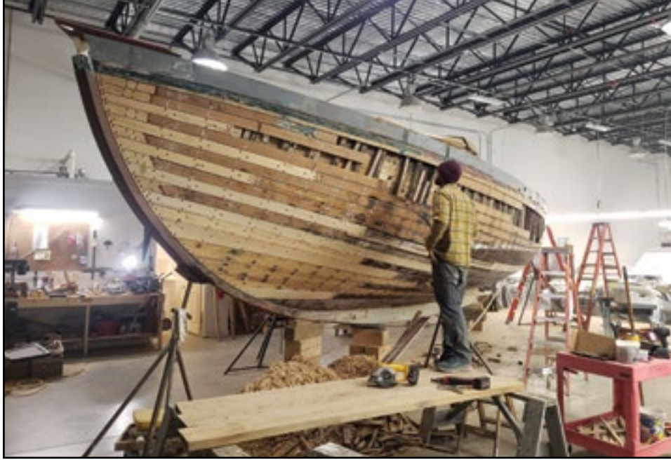
The Alden schooner being rebuilt by Richard Stanley and his assistant in Brunswick. The planking is nearly done and they are working on the chainplates.
