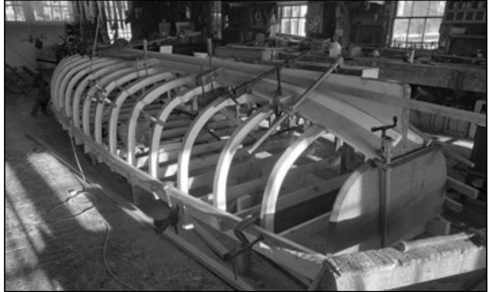
This is an Irish seine boat, which is under construction at Lowell's Boat Shop in Amesbury, Massachusetts. The customer is from Boston, but also has a place in Ireland where he has a small body of water to cross to get back and forth.
