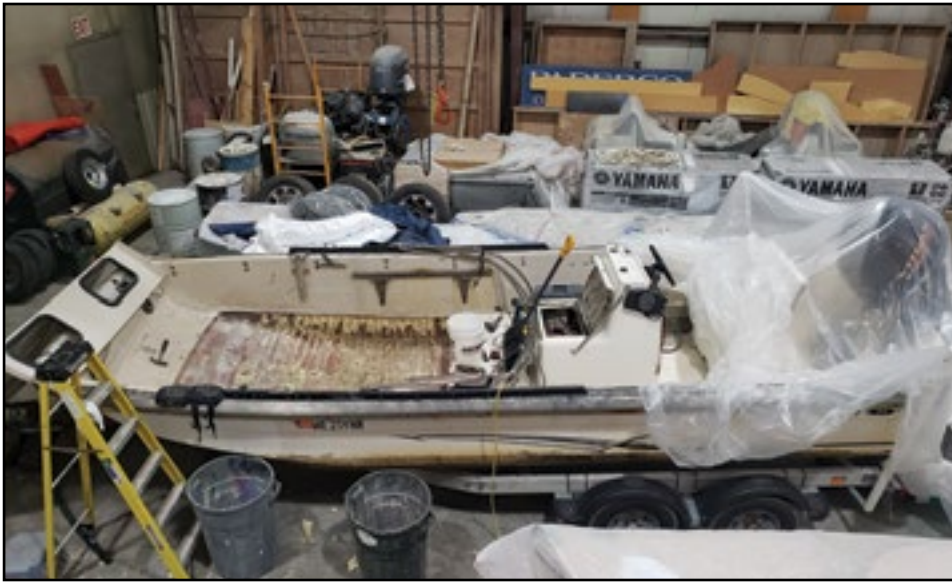
At Padebco Custom Boats in Round Pond they have removed the forward deck and the foam in this Carolina Skiff. They will be adding bulkheads to stiffen up the hull and then will put down a plywood deck covered with a heavy layer of fiberglass.
