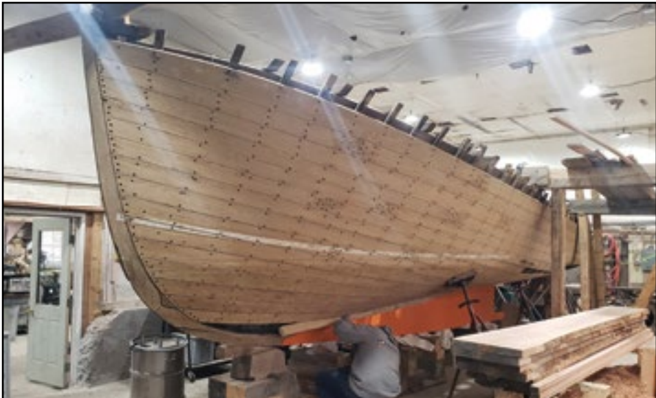
This is ROYAL, which is at Downeast Custom Boats getting rebuilt. The new keel is in and they are now getting ready to replace floors and frames as needed.
