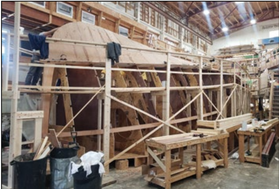
The 55-foot Wheeler is getting layers of plywood placed on the hull stations at Brooklin Boat Yard in Brooklin.
