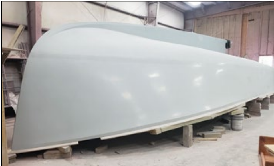
The new Libby 41 plug after some modifications and a lot of fairing is almost ready to take a mould off of at East Side Boat in East Machias.
