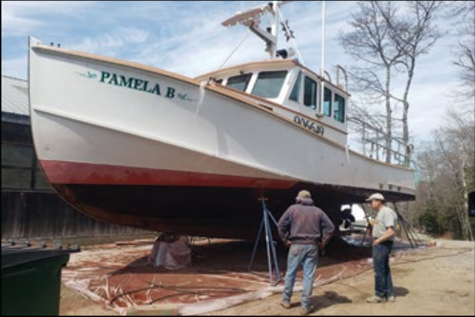
The hard-chine wooden lobster boat PAMELA B. owned by Jim Bartlett of Beverly sitting on the hard at Bittersweet Boat Yard in South Bristol. She has just had her bottom blasted by Aqua Terra Vapor Blasting.
