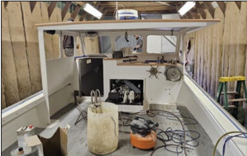
This is the second Stanley 36 from John Williams, Boatbuilder of Hall’s Quarry. She was given a major rebuild at Rich’s Boat Yard in West Tremont this winter. All that was left when they stripped her down was the V-berth and the platform. They are nearing the end as they paint the top of the trunk cabin.
