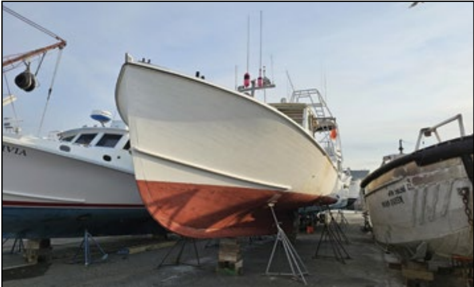
SARI ANN I is looking better. Ann and I have sanded the topsides and started putting coats of primer on. Hoping to get four coats of primer and two of final on her before she goes over.
