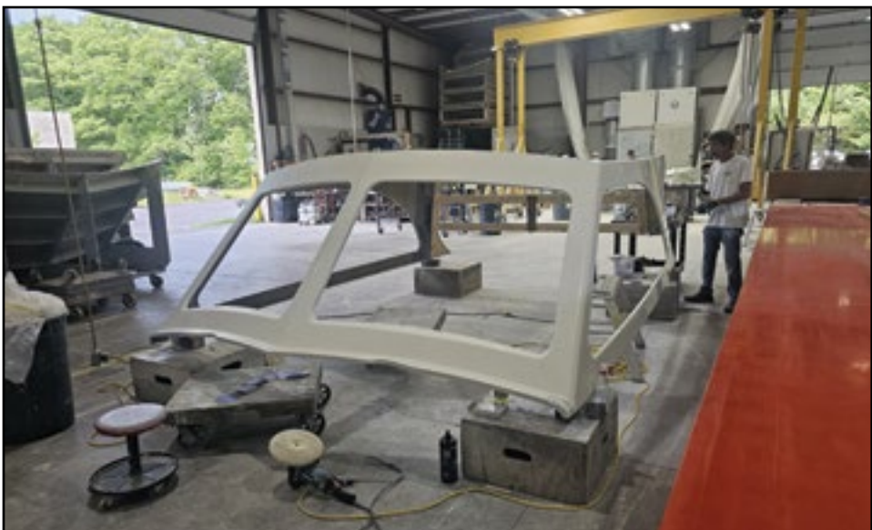
This is a windshield for a Hinckley powerboat, which is under construction at Custom Composites in Bath.
