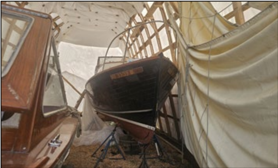
This is a Hodgdon 27 having some repair work down at Newcastle Marine/ Blood Boat Works in Newcastle. They have repaired the aft end of the keel and have now just replaced the cockpit deck.
