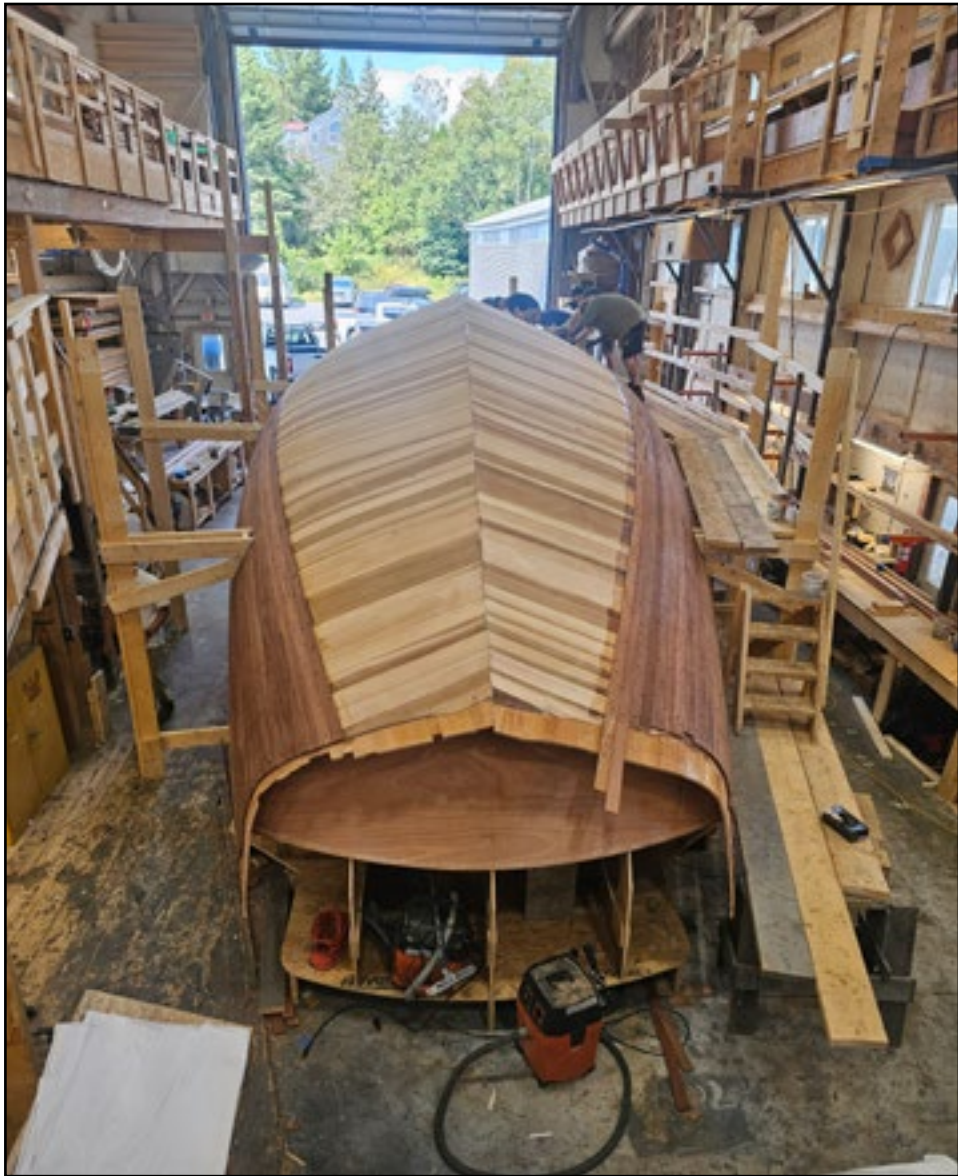
At Brooklin Boat Yard in Brooklin they are putting on the layers of wood for this cold moulded hull of a 56-foot sailboat.
