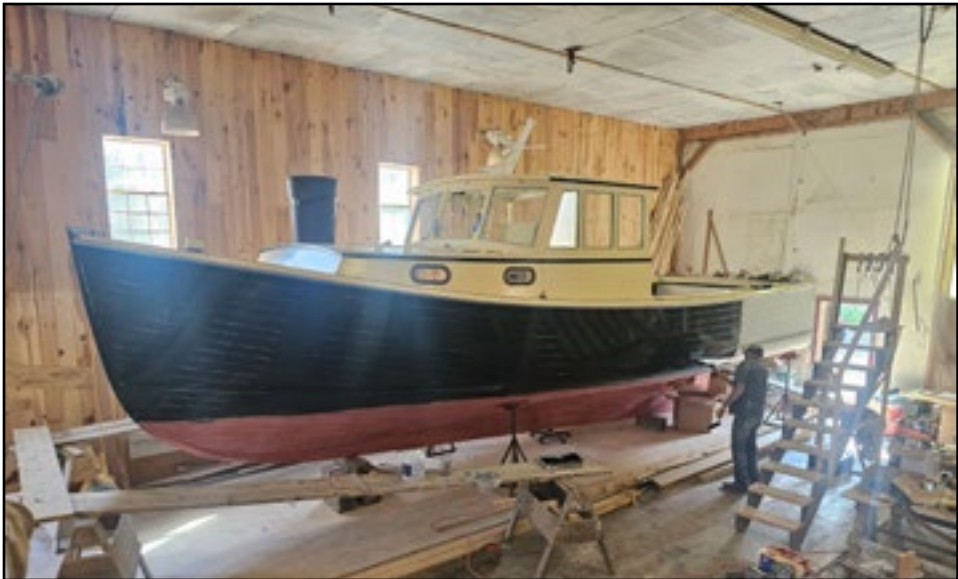
Peter Buxton of Buxton Boats is applying the final coat for the topsides of this 32-foot lobster yacht. She will be launched the second week of September.
