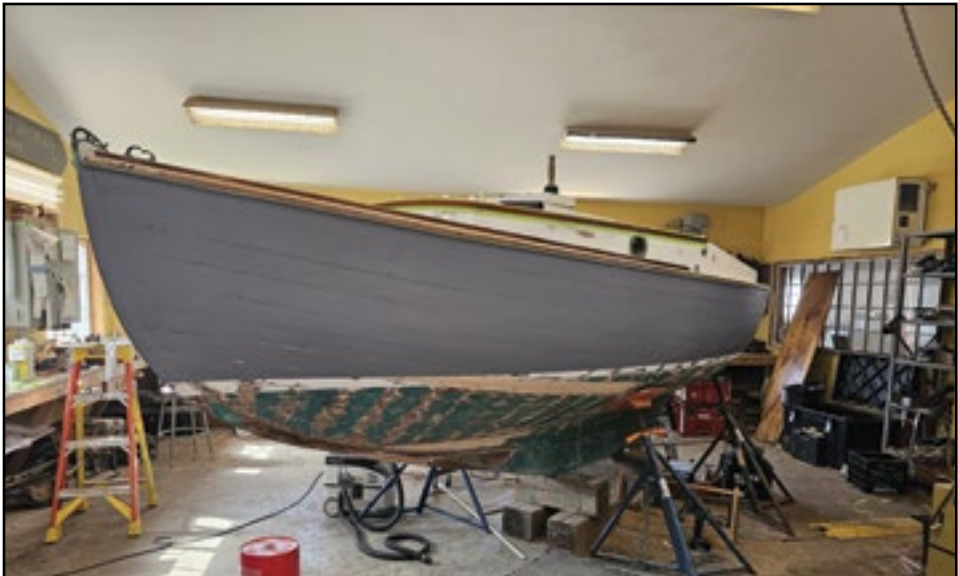
Artisan Boat Works in Rockport are making repairs to SEA LADY, an Aage Nielson double-ender. They did the stern a couple of years ago and this year the front half got rebuilt.
