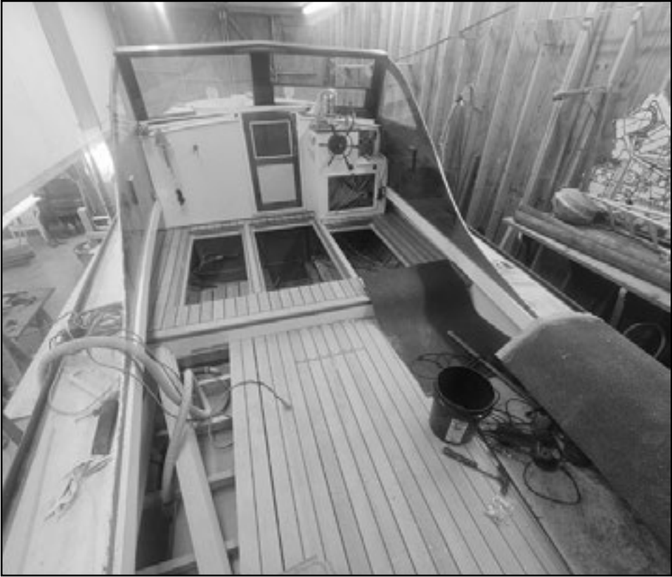
Wayne Rich of Bernard has kept himself busy this winter. This boat was built by Henry Barnes of Harpswell in 1959. They have made repairs to the bow, refastened the bottom, and replaced the platform. She will be ready for the water later this spring.
