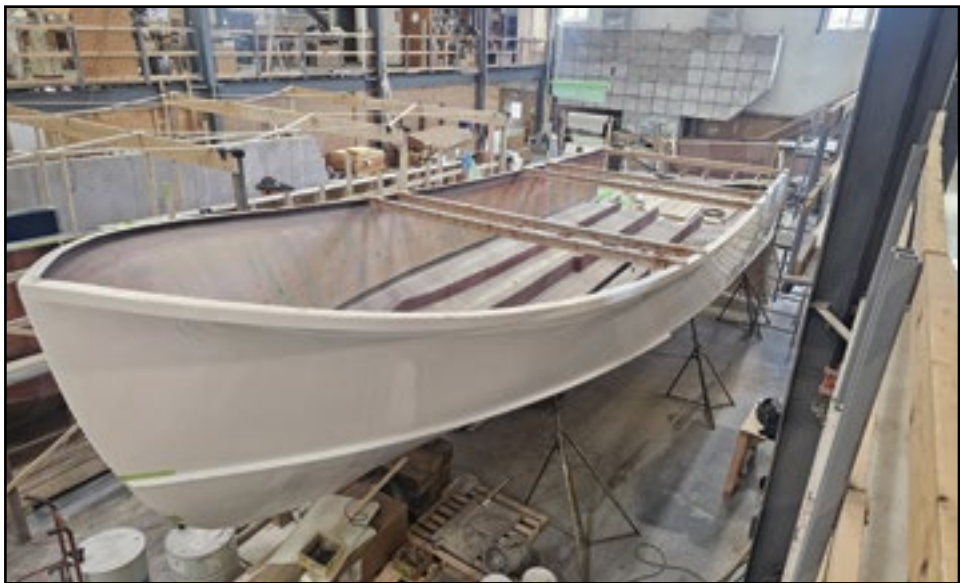
This is a Wesmac 42 getting a four-foot extension at Front Street Shipyard in Belfast. She will be finished off as a walk-around cruiser.
