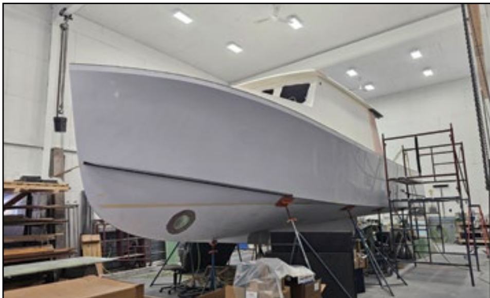
This is a Mussel Ridge 42 under construction at Samoset Boat Works in Boothbay. She is pretty far along, with her engine and drive train in as well as much of her accommodations.
