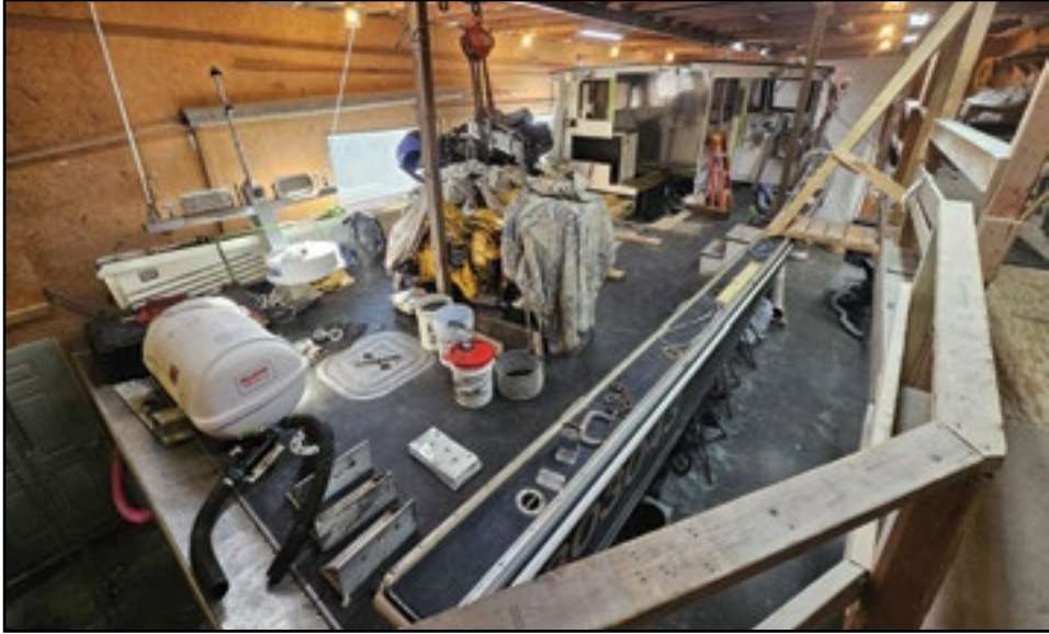
The Young Brothers 45 MISS QUAHOG in at Farrin's Boat Shop in Walpole to be re-powered. They have removed a 700-hp John Deere and will replaced with a 1,000-hp FPT.
