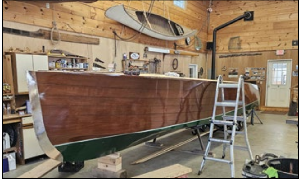
This is a 1924 Chris Craft getting restored at Woodman Boats in Kennebunkport. They were able to save a lot of the planking, but had to repair it. She has been given a new bottom and they are now working on the deck.
