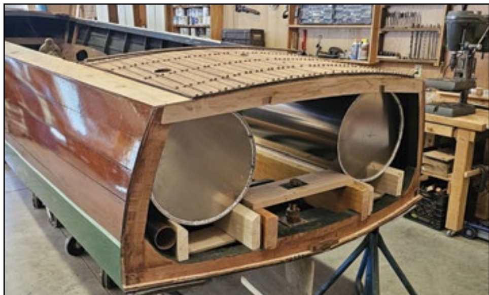
A stern view of the 1924 Chris Craft getting restored at Woodman Boats in Kennebunkport. Note the two large fuel tanks being fitted as well as the old deck being re-laid.
