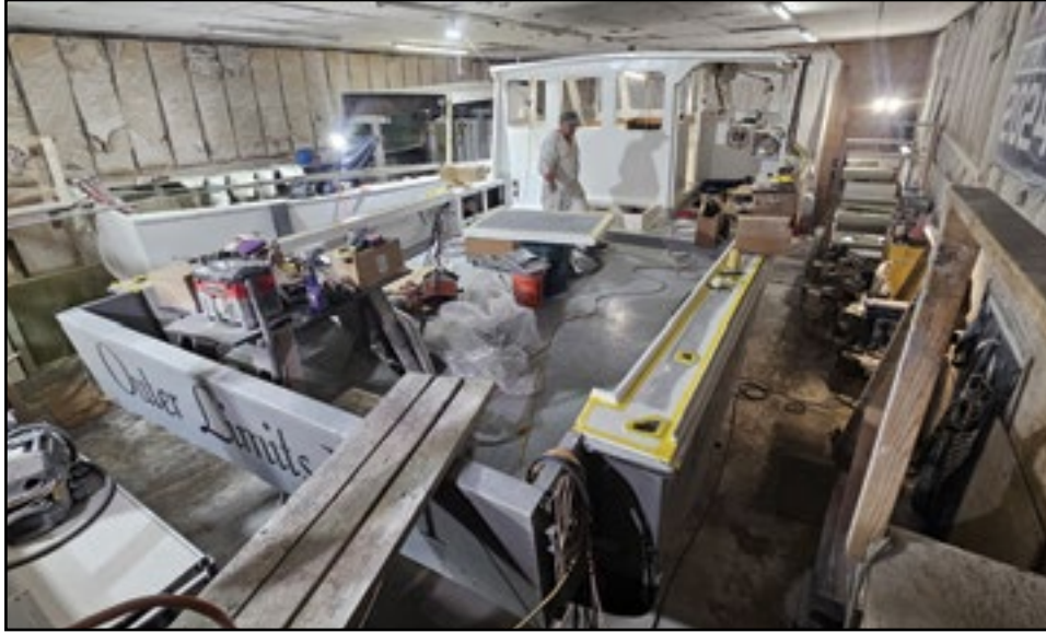
This is the lobster boat OUTER LIMITS in to be repowered and other upgrades at Mainly Boat in Cushing. They have removed a 600-hp Cummins and replaced it with a 815-hp FPT.
