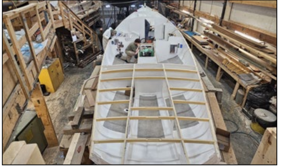
The Eggmoggin 47 under construction at Brooklin Boat Yard in Brooklin. Note the deck framing is in along with several bulkheads and the engine.
