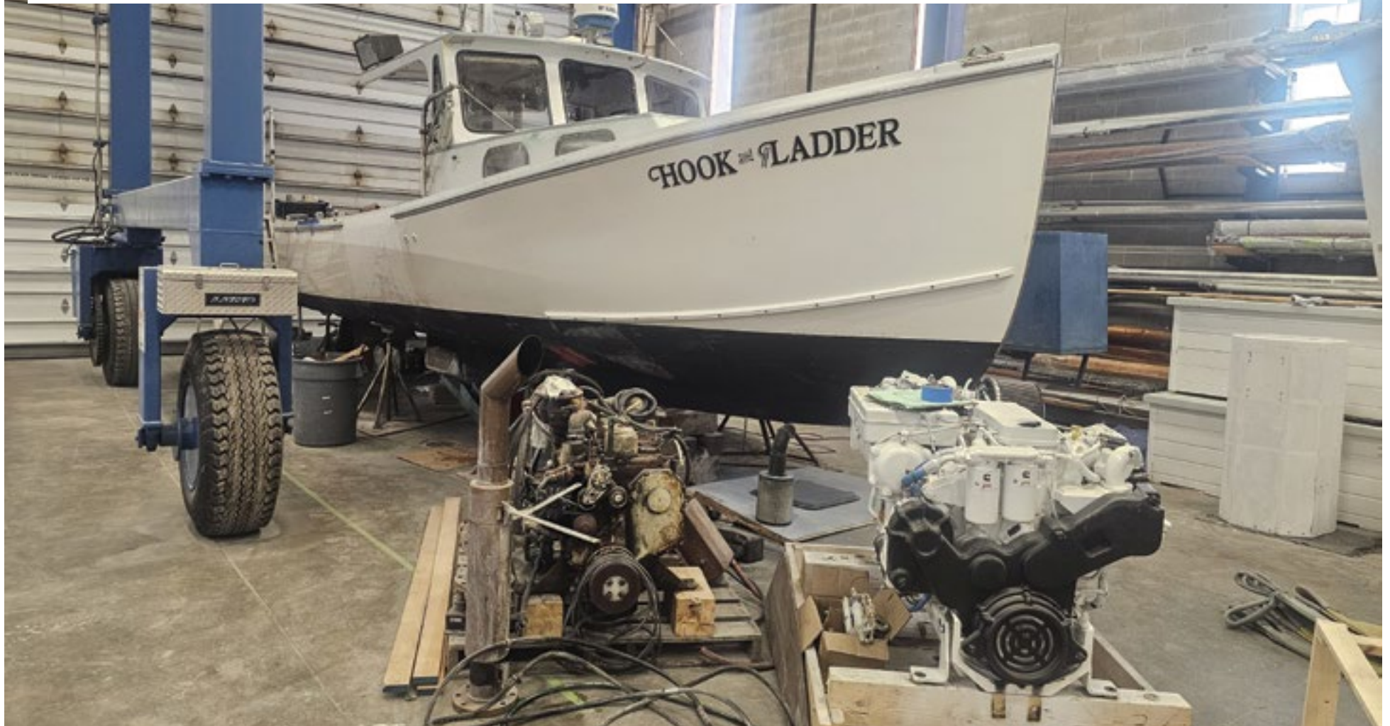
This Holland 30 is getting repowered and upgraded by three students at Maine Maritime Academy in Castine. In the foreground is the original 210 being replaced by a 485-hp Cummins.
