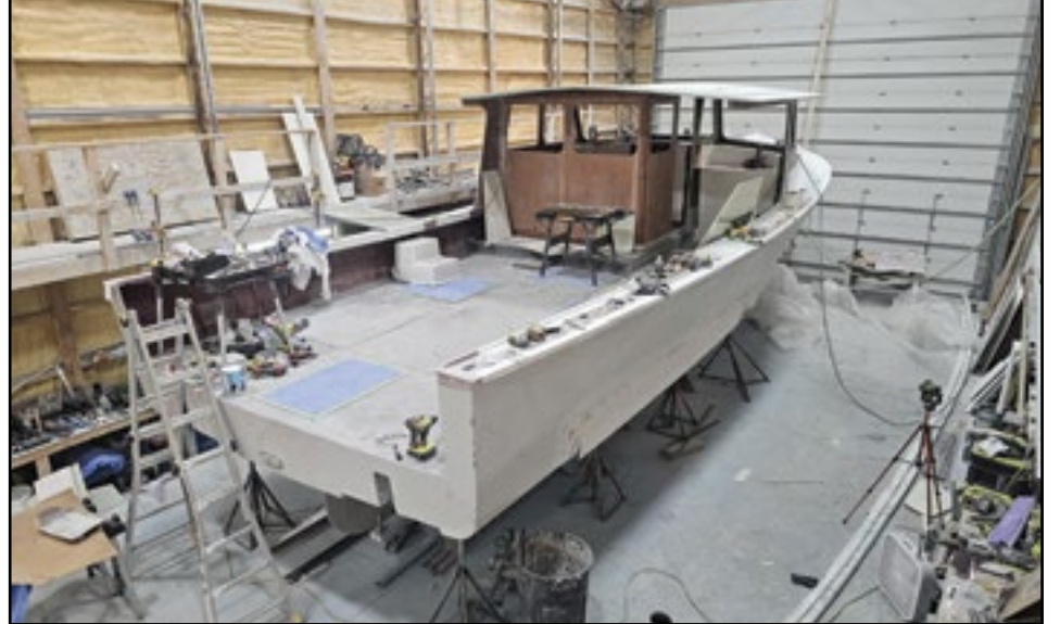
In the far bay is a Wayne Beal 36, which is being finished out as a split wheelhouse lobster boat at A. R. Kennedy Custom in Steuben.
