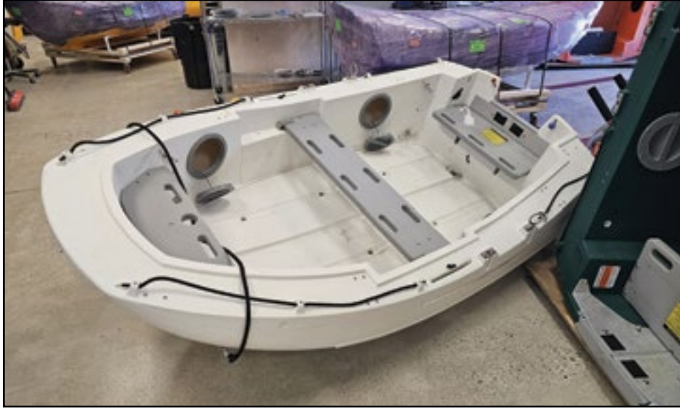
This is a Portland Pudgy, which is 7 feet 6-inches in length and can be rowed, sailed or powered with an outboard. They are built in Biddeford.
