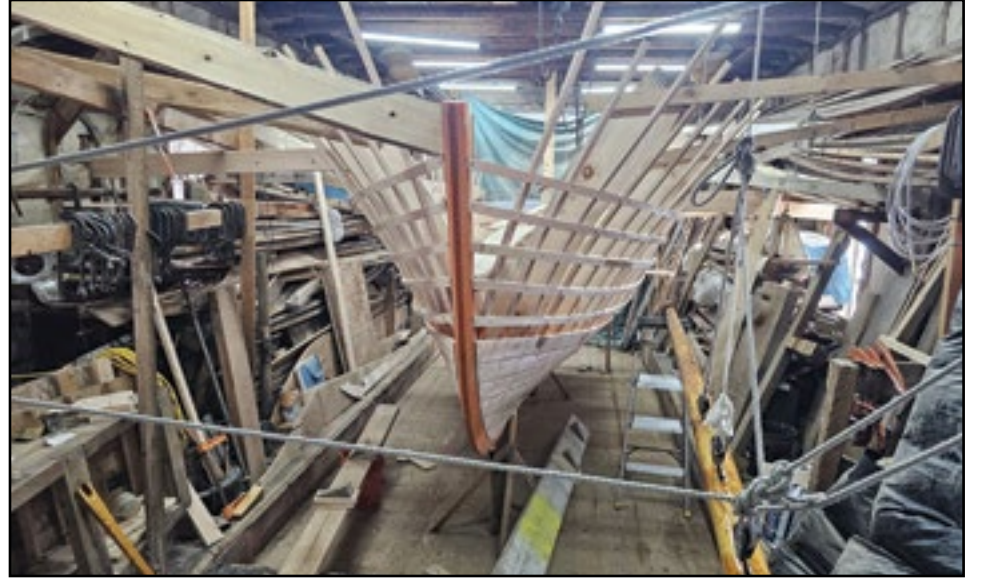
This is a 21-foot Striper, under construction at Riverside Boat in Newcastle. She is halfway planked, but she is on hold while yard workers get the storage boats ready for the water.
