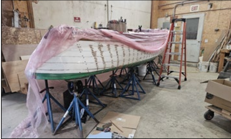
A Fay & Bowen launch from 1906 being rebuilt at Hylan & Brown in Brooklin. They have replaced frames and part of her keel and added an electric pod.
