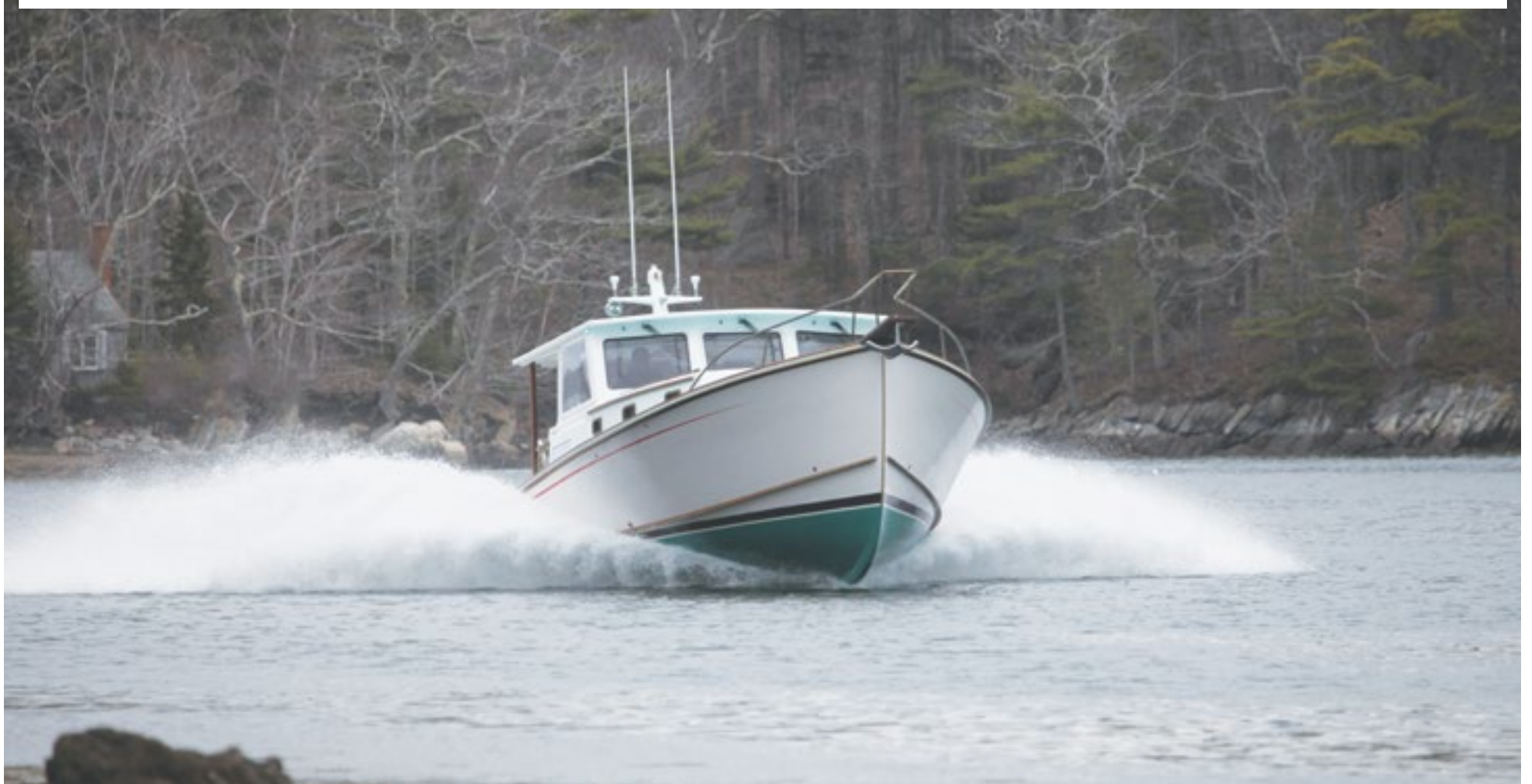
Farrin's Boat Shop of Walpole doing sea trials on the new JANA B. of Kingstown, Saint Vincent and the Grenadines in South Bristol on 22 April. She is a Young Brothers 40 finished out as a sportfish boat powered with a 725-hp Volvo Diesel.
