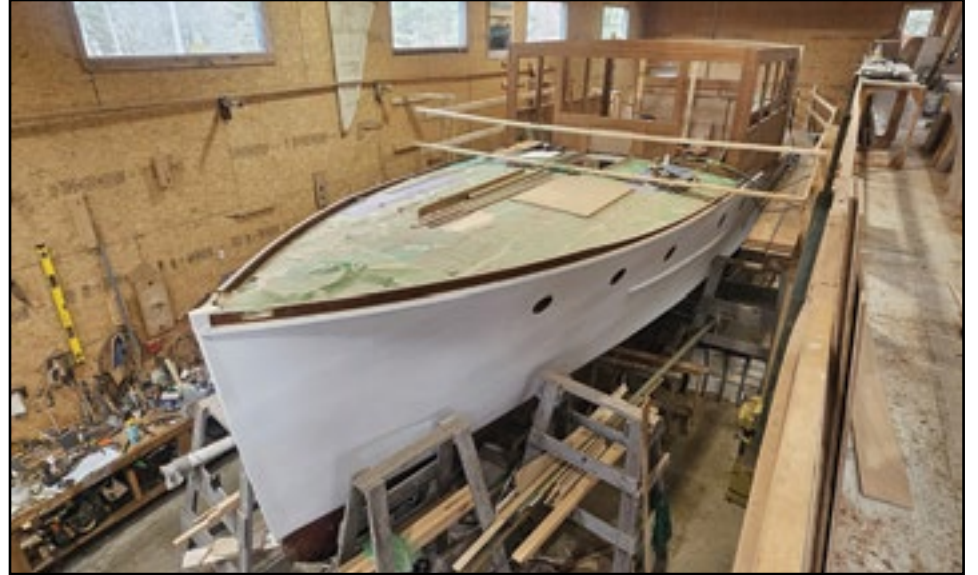
This is an Elco cruiser which has been under a rebuilding program for a number of years at Hylan & Brown in Brooklin. She is in the final stages, but probably needs another winter.
