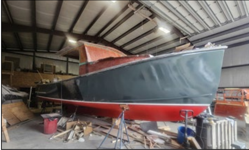
This boat suffered from balsa core issues, which were being repaired at Friendship Boat Works in Friendship. The house has been replaced with plywood covered with fiberglass.
