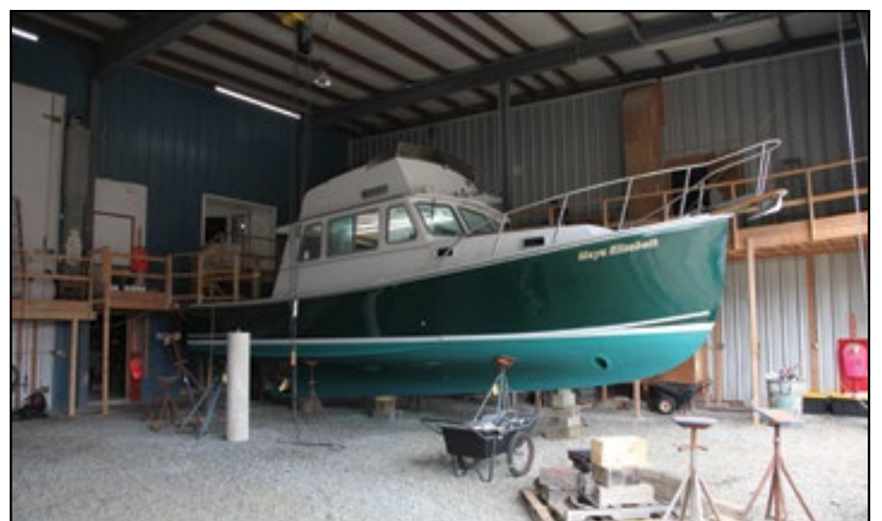
MAYA ELIZABETH, a Duffy 35, was repowered with a C7 Caterpillar, new Northern Lights generator, AC/heat units and wiring upgrades. She will be going over in early June.
