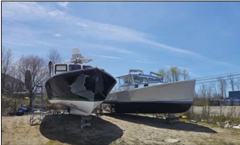
Two boats at Jeremy Beal's shop in Jonesport. The one to the left has major issues as all her bulkheads have come loose and they were awaiting the insurance company's for a decision.
