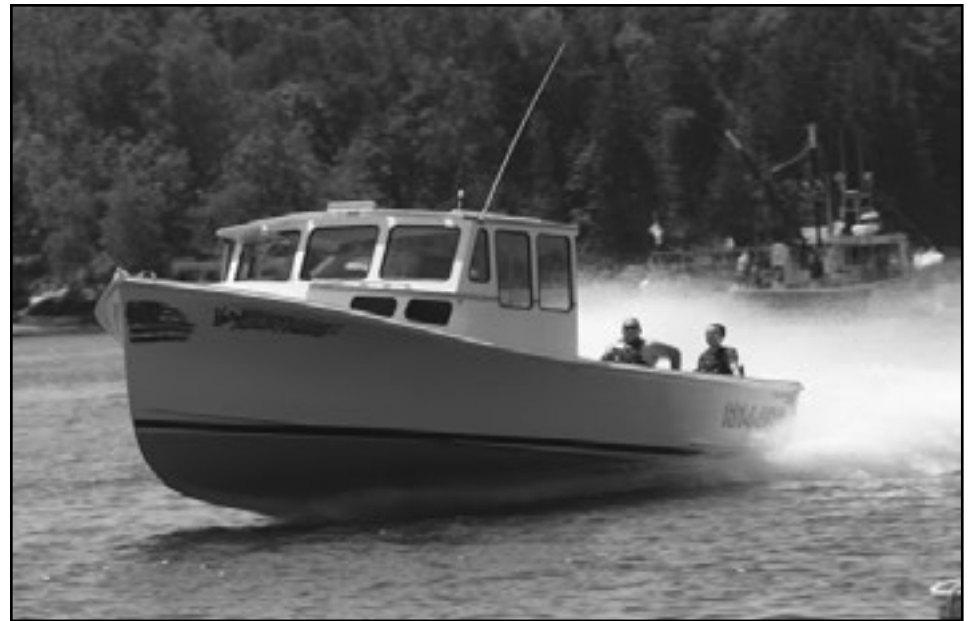
This is a Wayne Beal 32, powered with 1,000-hp Isotta, capable of speeds over 65 mph.
