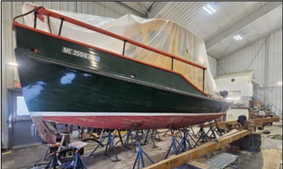
A small wooden tugboat having her keel replaced at Yankee Marina in Yarmouth. The keel has been removed and you can see the new one in the background.
